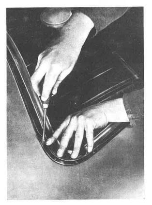
2. Fasten, but do not tighten, the hood to the hinges and adjust in the slots until the panel fits with equal clearance all around. Tighten screws
